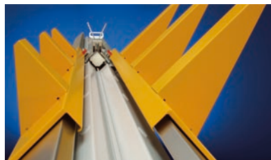
The RAS material handling system with short front and long rear arms to support the duct.
