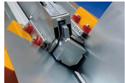
The reinforced DuctZipper RAS 20.12 seaming bar
