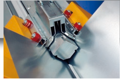
The DuctZipper RAS 20.10 seaming bar
